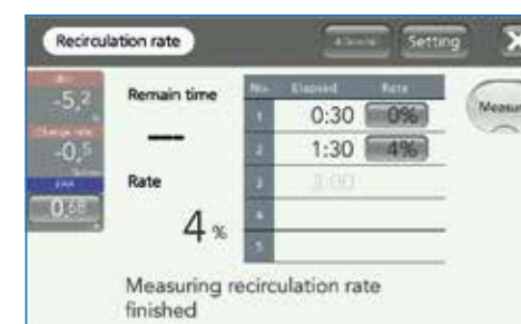
Recirculation rate - Schedule and results
